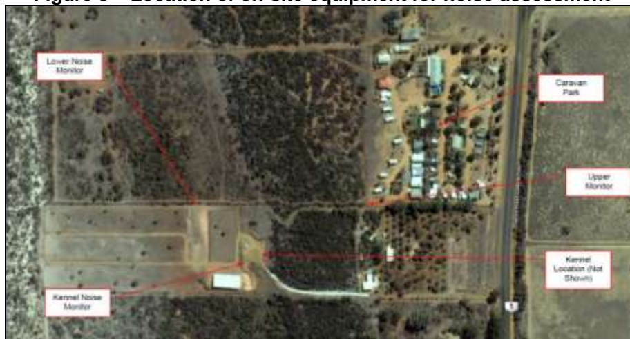
Figure 8 – Location of on-site equipment for noise assessment
