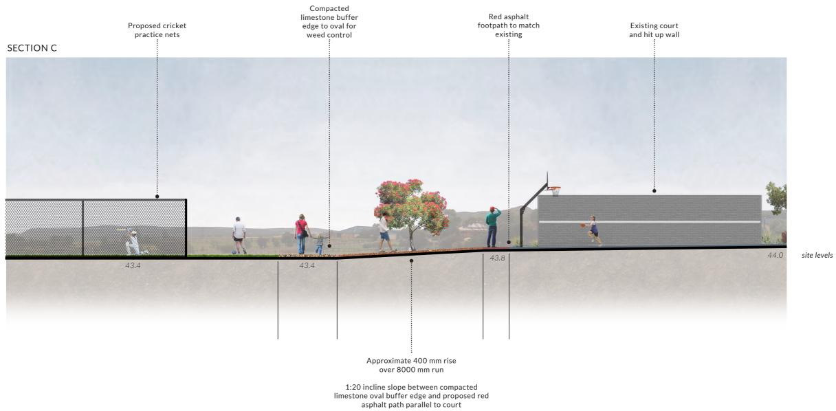
Slope to be evenly graded with compacted gravel to match existing boundary track
