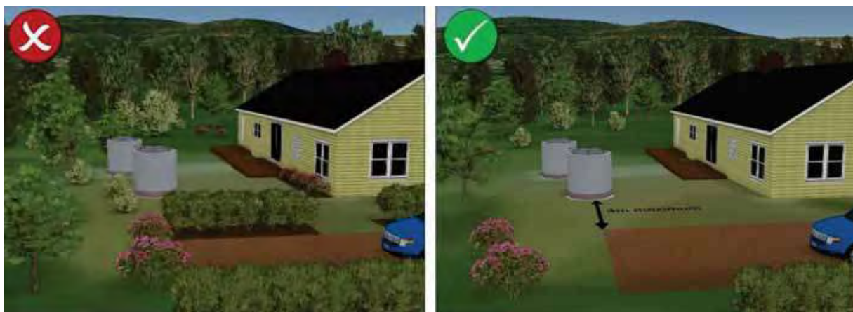
Figure 30: A good and bad example of landscaping around a water tank
